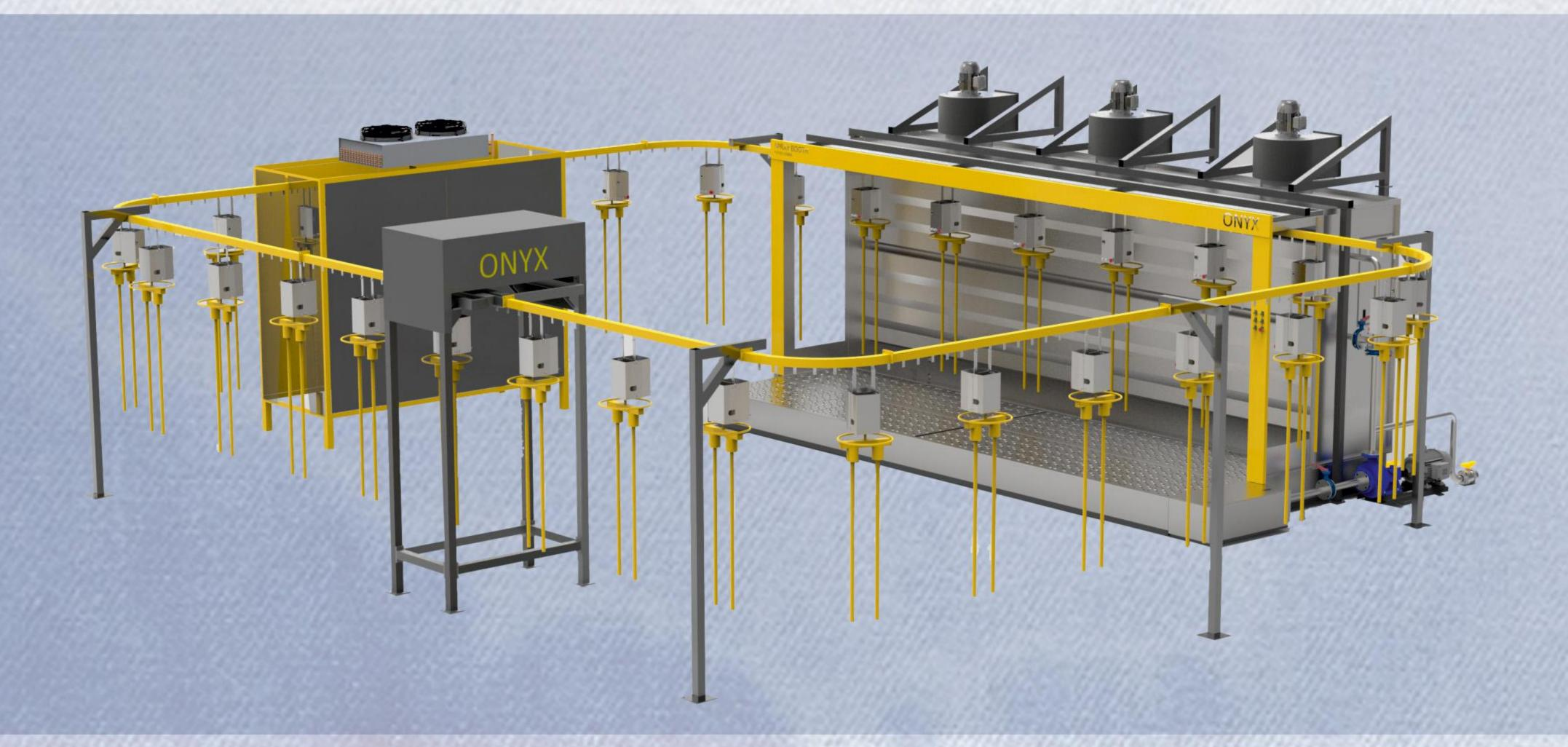
Specially designed Spray booth with conveyor and Hot chamber for Higher Production.
